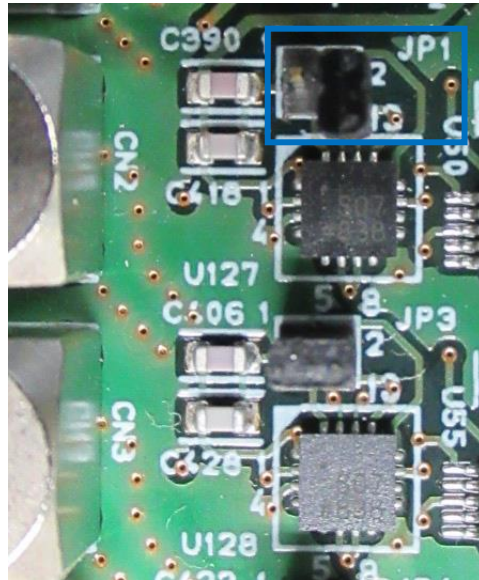
Picture 7 APV8016A5 base board CH1 input section
