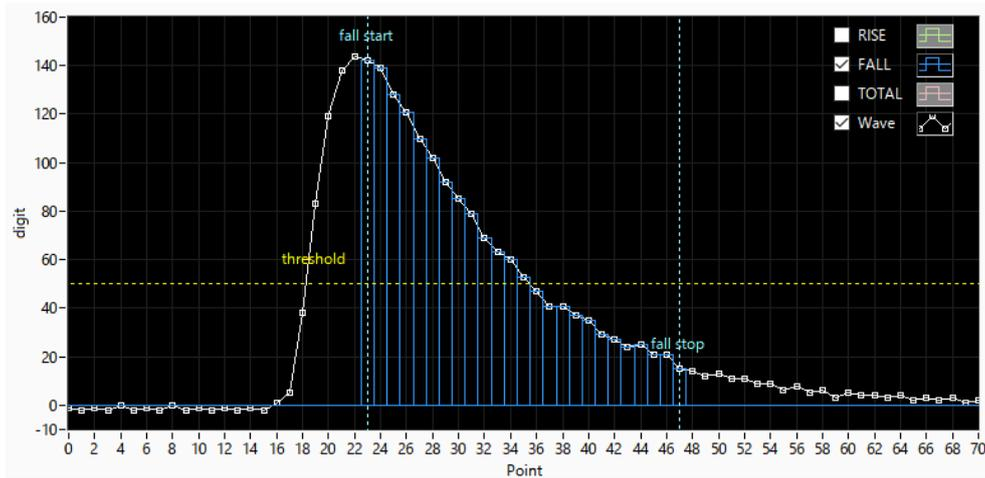
Fig. 4-2-3 How to calculated FALL value
