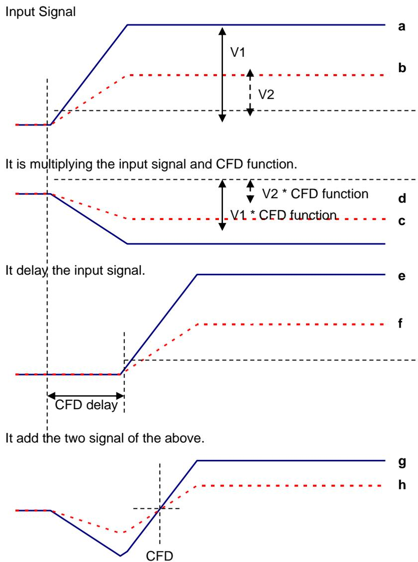
Fig. 4-2-3 How to use Constant Fraction Discriminator Timing
