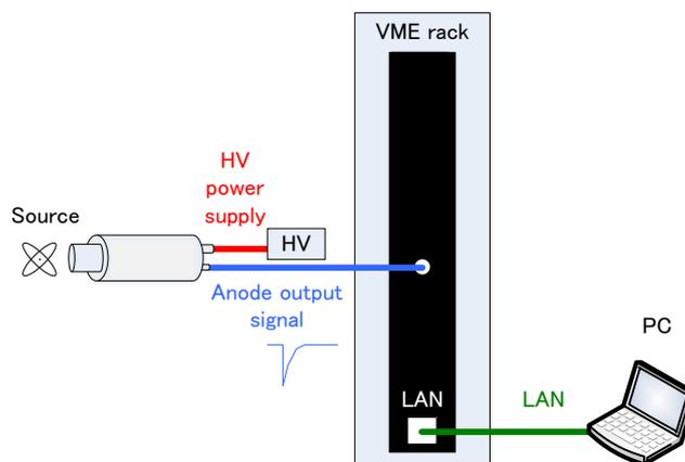
**Experimental environment of energy spectrum measurement**
