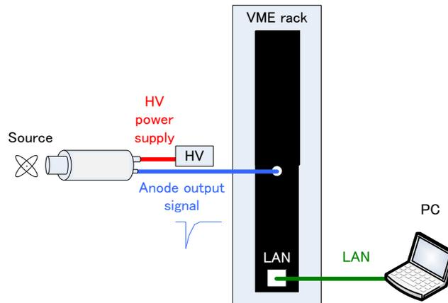
**Experimental environment of energy spectrum measurement**
