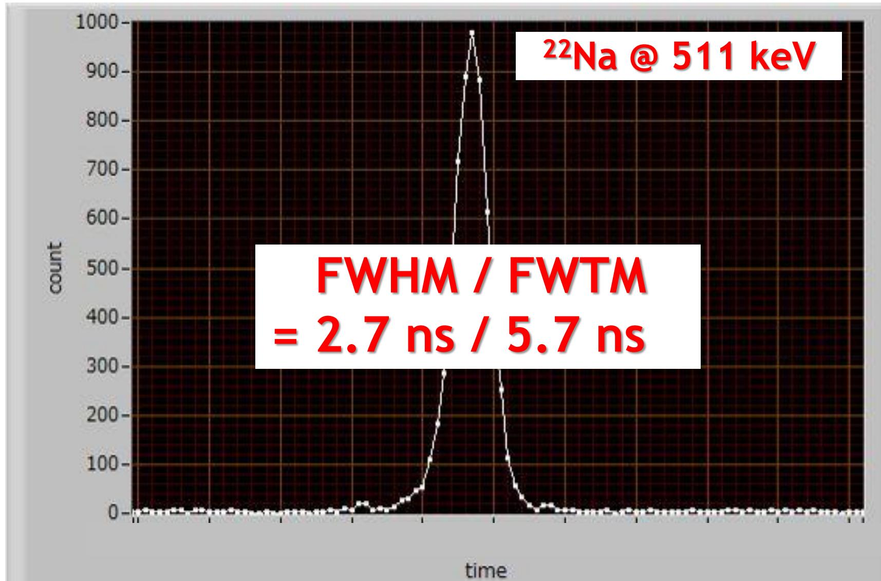
The time resolution of the GSO scintillation detector
