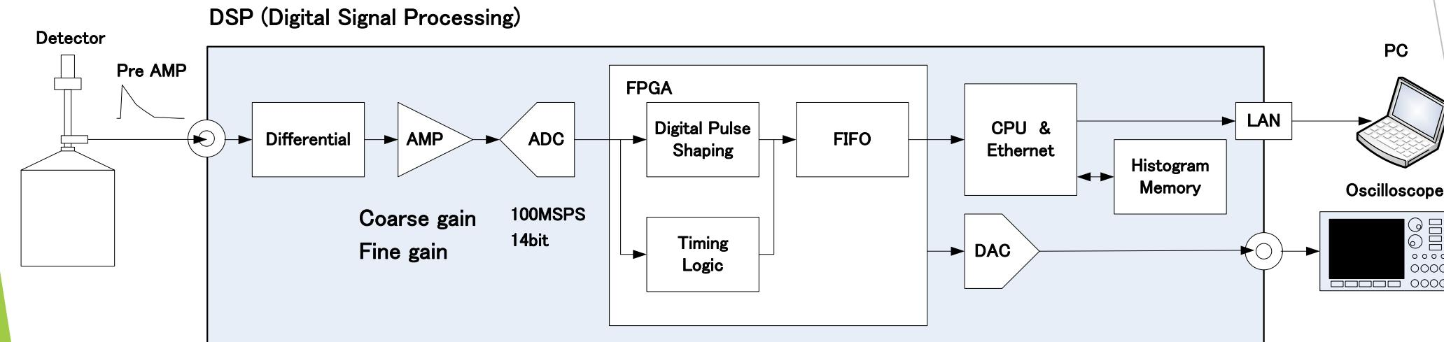
**Block diagram of the DSP circuit board**
