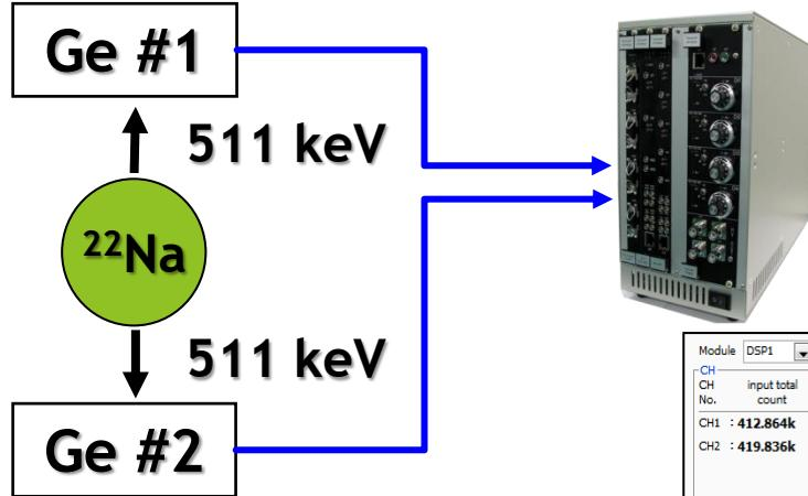
It is able to support the coincidence processing using several detectors.
