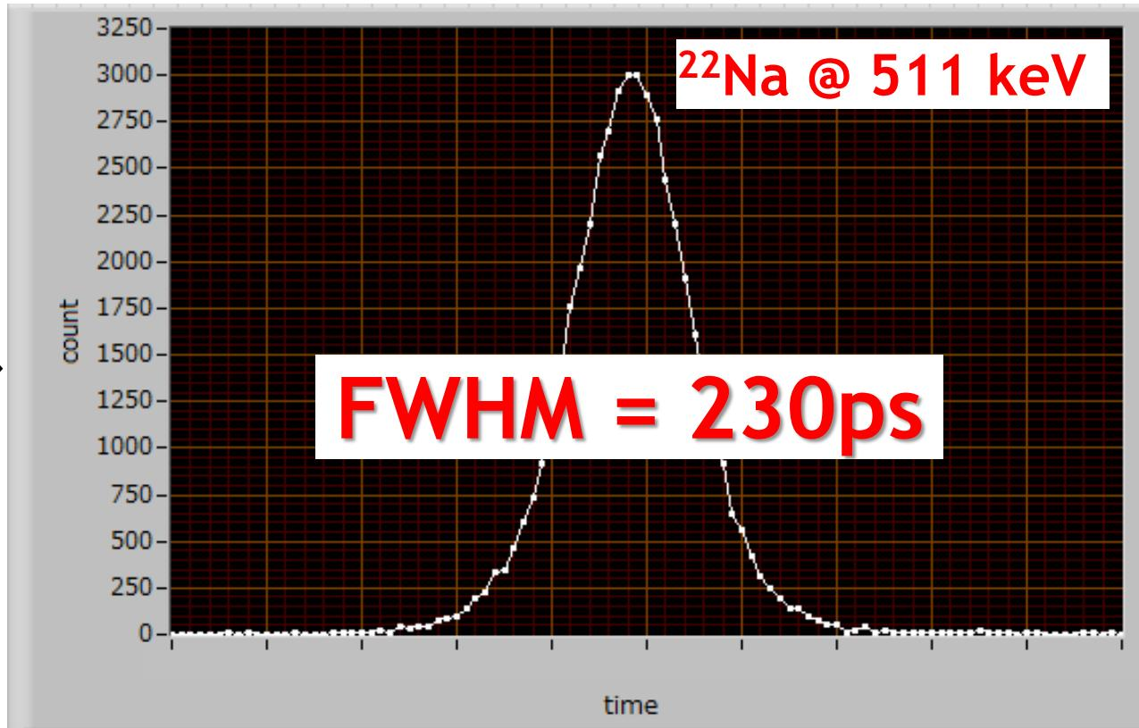
LaBr<sub>3</sub>(Ce) scintillation detector
