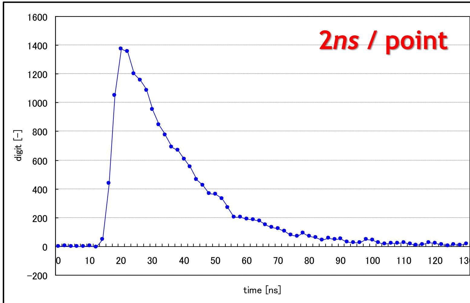
LaBr<sub>3</sub> @ 662 keV (<sup>137</sup>Cs), The sampling interval is 2ns.
