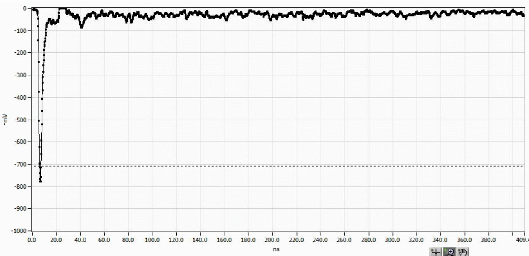
BaF<sub>2</sub> @ 511 keV (<sup>22</sup>Na), The sampling interval is 0.2 ns.
