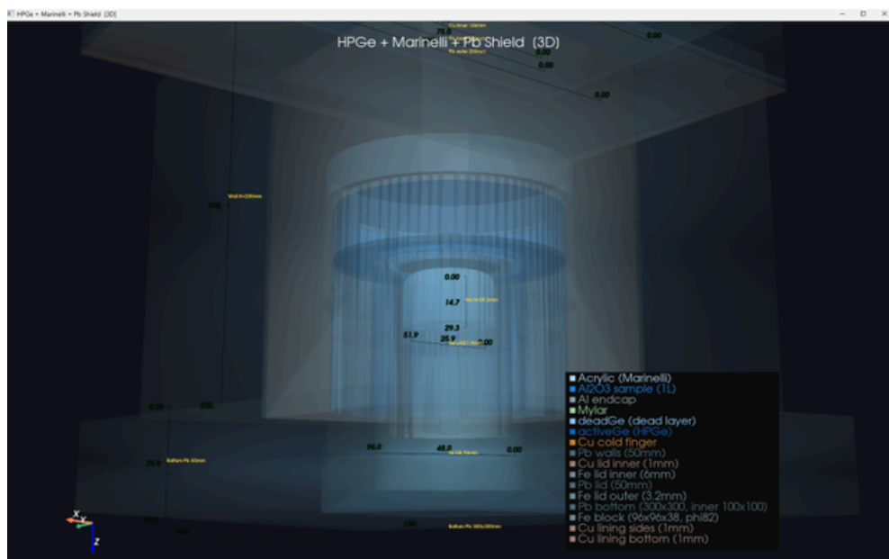
Geant4 HPGe geometry Marinelli 1L
