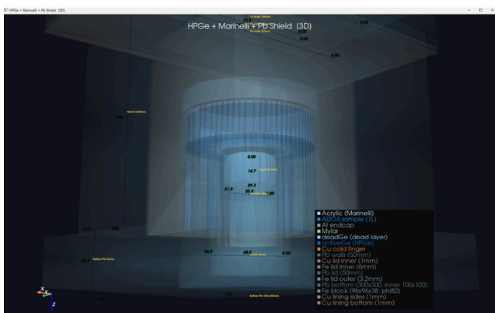
Geant4 HPGe geometry Marinelli 1L
