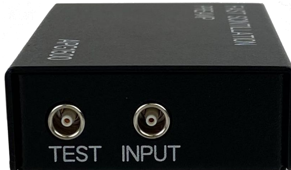
Picture 3 INPUT connector and TEST connector
