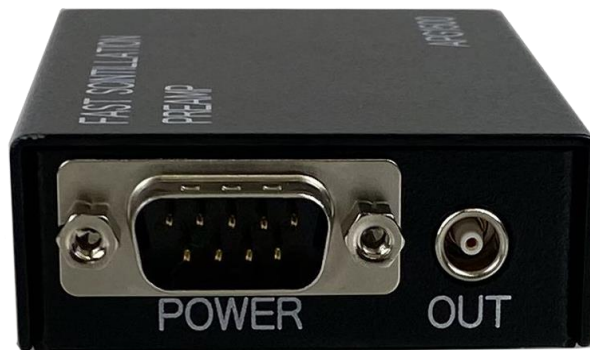
Picture 4 POWER connector and OUT connector
