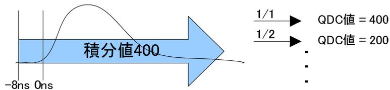
**QDC LLD (digit)** Sets the LLD (Lower Level Discriminator) of the QDC. The unit is digits. Set a value smaller than ULD. The setting range is from 0 to 8191.
