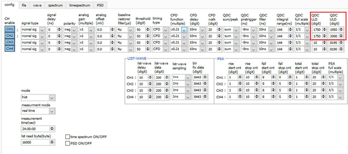
Figure 33 Energy spectrum measurement before time spectrum measurement (energy range narrowing setting)
