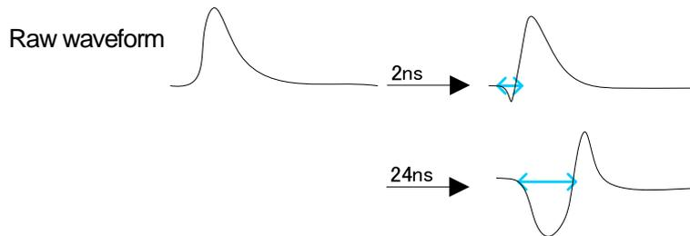
**CFD walk** Sets the threshold value to be time-stamped. The unit is in digits, and the value is set near the 0 crossing position while watching the CFD waveform in wave mode.
