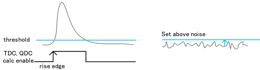
Constant Fraction Timing of APV8104 and APV8508 is realized by digital signal processing using FPGA
