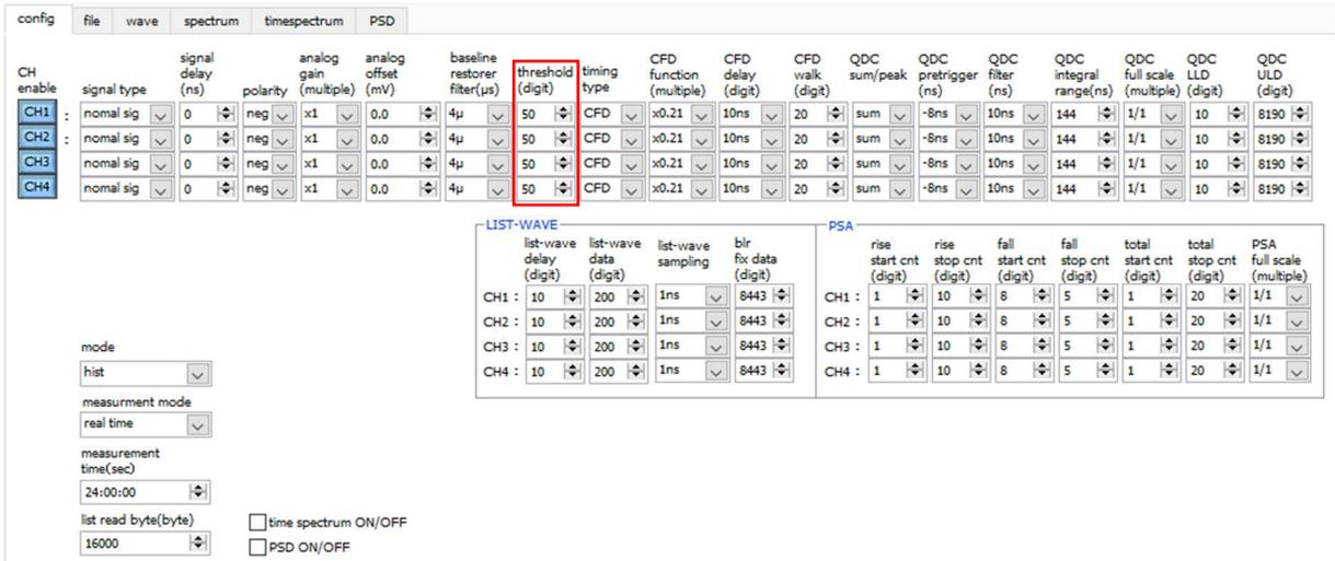
Figure 25 Threshold setting in config tab
