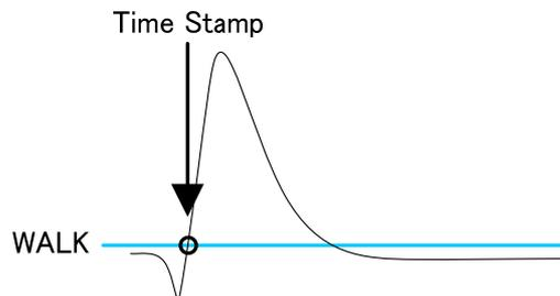
**QDC pre trigger (ns)** Selects the timing to start waveform shaping for integral value calculation from 0ns, -8ns, -16ns, -24ns, -32ns, -40ns, -48ns, -56ns, and -64ns.
