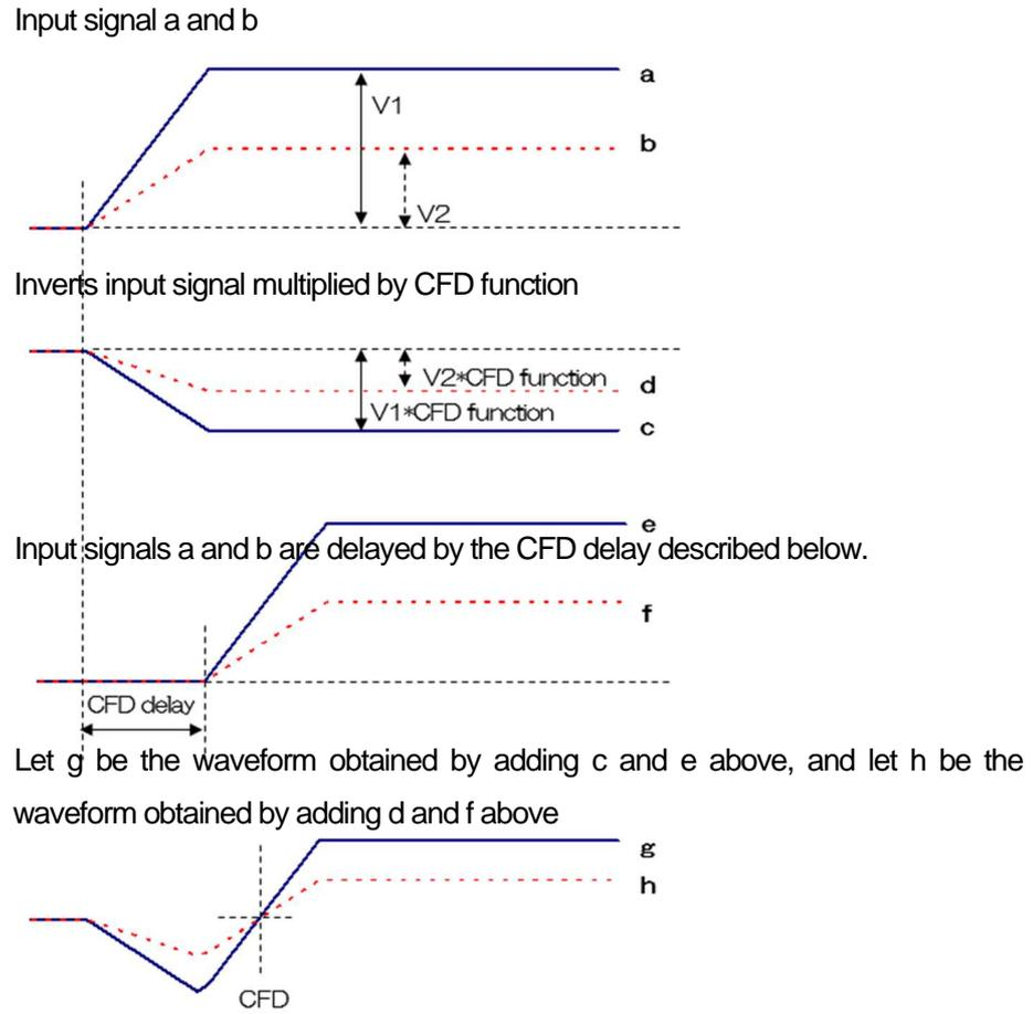
Figure 6 Thinking of Constant Fraction Discriminator Timing
