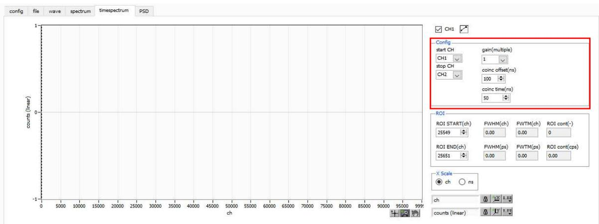
Figure 36 Time spectrum measurement settings in timespectrum tab
