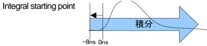
**QDC integral range (ns)** Set the QDC integration time from 48ns to 32000ns in 8ns increments
