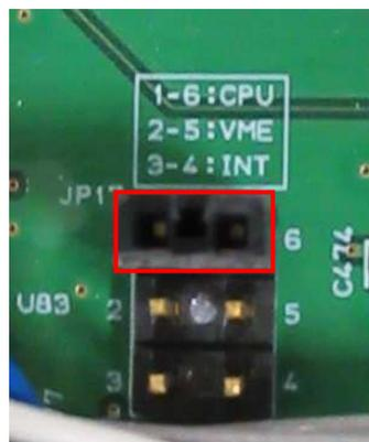
Photo 5 External clock operation (1-6: CPUjumper)
