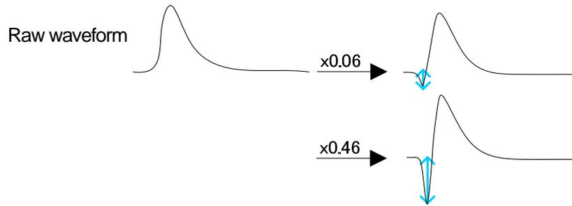
**CFD delay** Sets the CFD delay time; for the APV8108, set from 1ns to 16ns in 1ns increments
