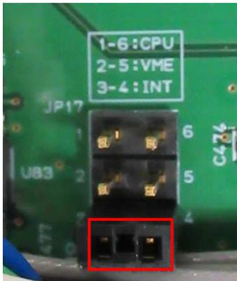
Photo 4 Internal clock operation (3-4: INT jumper)
