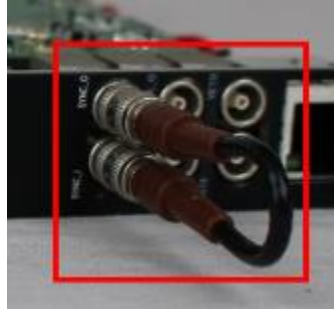
Photo 2 Interconnects SYNC-O and SYNC-I terminals
