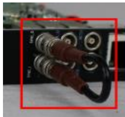
Photo 3 Example of SYNC-I/O terminal connection
